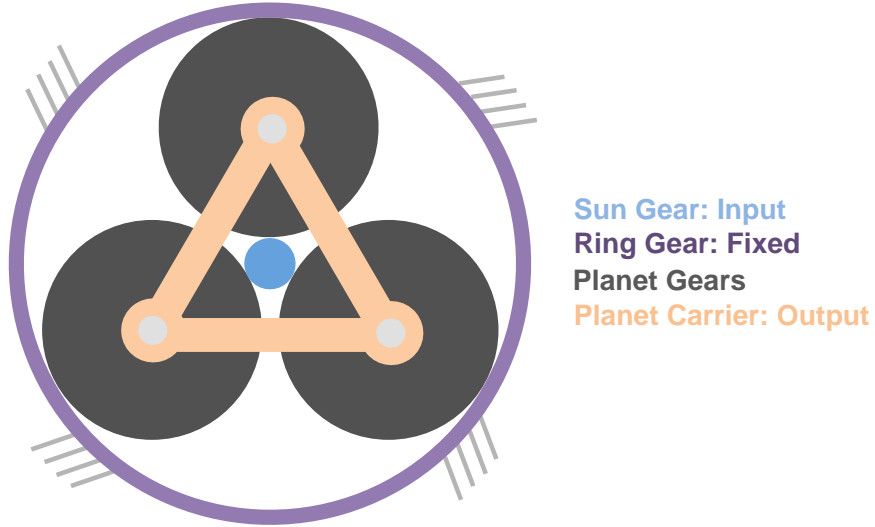
Figure 2.10: The ideal configuration for maximizing reduction of a single-stage planetary gear is to fix the ring gear, couple the sun gear to the motor input, and the planet carrier to the output. Circles represent the gear's pitch radius so teeth are not shown.
