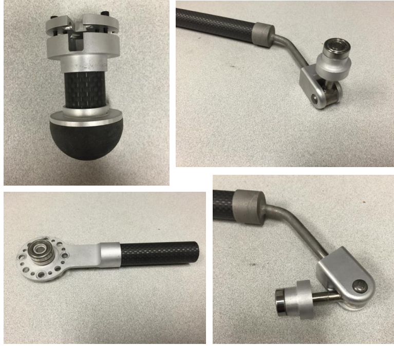
Figure 3.15: Various mechanical components of the 3-RSR leg including foot, knee, and driven link l_1 .
