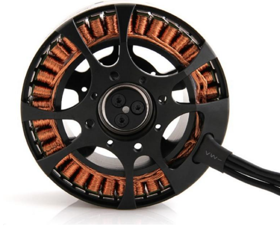
Figure 3.16: The Tiger Motor U10 shown here has a large 40 mm gap radius and a lightweight frame. The T-motor U8, U10, and U12 were determined to have one of the highest thermal specific torques of any COTS motor ( 0.42 \frac{Nm}{kgC^\circ} at r_{gap} = 40 \text{ mm} ) [43]. For reference the custom MIT cheetah motors have a thermal specific torque of 0.71 \frac{Nm}{kgC^\circ} at r_{gap} = 49 \text{ mm} [9].
