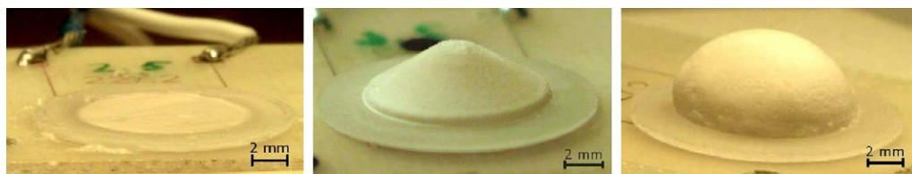
Fig. 53. Photographs showing the paste (a) unexpanded (state before actuation), (b) expanded (state after actuation; liquid container removed for visualization) and (c) expansion without constraining liquid container results in a volume expansion of seven times the original volume.
