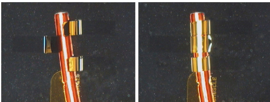
Fig. 61. Three bilayer actuators (500 \mu\text{m} wide) grabbing a 0.5 mm wire.
